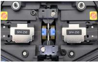
Close the cover. Splicing will start automatically if the pause settings for alignment and focus are disabled (default setting). Otherwise, press to start splicing.
