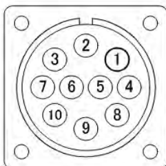
(View of terminal on instrument)
