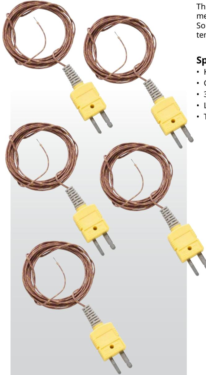
This K-Type thermocouple is designed for temperature measuring applications and is compatible with Fluke Solmetric SolSensor. The thermocouple can be used to measure temperature range from 0 °C to 482 °C (32 °F to 900 °F).
