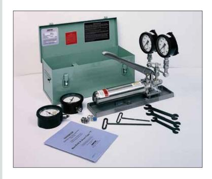
The AMETEK Comparators are ideal secondary standards for pressure measurement. The comparator test set consists of a hydraulic hand pump on a pan as the pressure source, a test manifold and a set of four 4.5 inch test gauges. Gauge PSIG spand vary with model.
