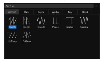
The USB waveform generator can output waveforms with up to 50 MHz frequency and ±3 V amplitude. Six basic waveforms together with multiple types of predefined waveforms and as user-defined arbitrary waveforms are supported.
