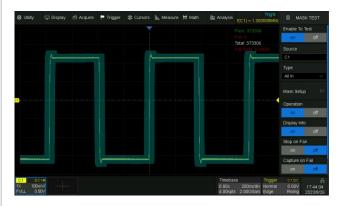
The oscilloscope utilizes a hardware-based Mask Test function, performing up to 14,000 Pass/Fail decisions each second. It is easy to generate userdefined test templates to provide trace mask comparisons, making it suitable for long-term signal monitoring or automated production line testing.
