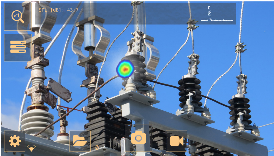
The FLIR Si2 camera detecting and locating partial discharge.
