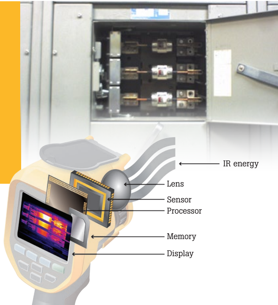
Figure 1. Anatomy of an infrared camera
