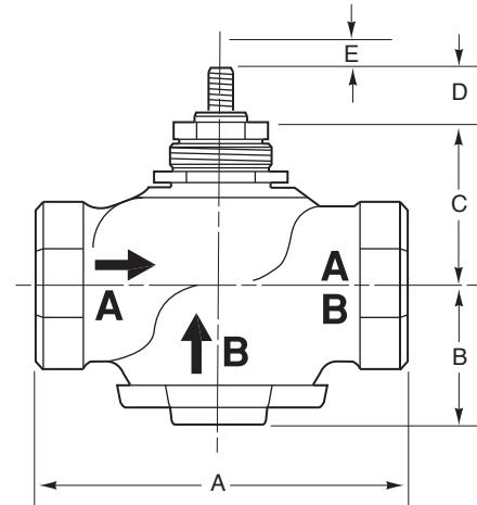
Note - VB-7253-0-4-P, VB-7273-0-4-P up normally open valves have inverted A, B, and AB port embossings
