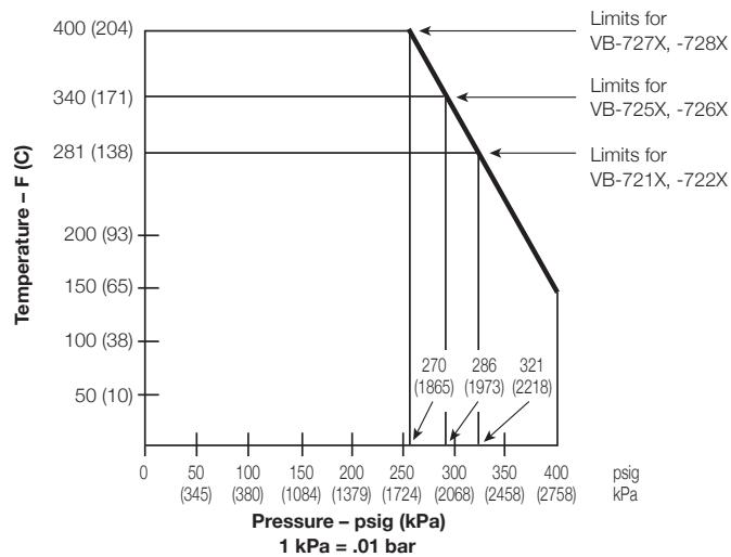
Caution: Do not use valves beyond rating of piping system and components. Consult ANSI B16.22 for ratings of solder joint pressure fittings.
