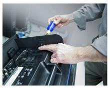
**6.** Place the oscilloscope on the base plate flush with the face plate. The screen should be fully visible and the front bezel should extend slightly past the face plate when seated properly.
