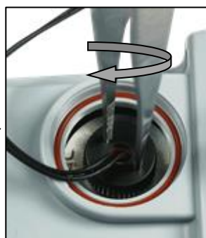
Close the lamp cover and screw tight with a tweezer.
