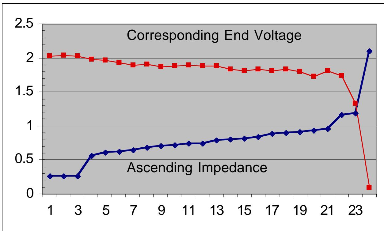
This graph shows ascending impedance with corresponding end-of-capacity voltage. It clearly shows a solid correlation between impedance and capacity. This graph is of an actual telecom battery. We know for example that the lowest three cells were recently replaced while the others date to the original installation.
