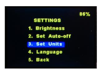
Press UP or DOWN to highlight the feature to be modified and MENU to access the next screen. Highlight BACK and press MENU to return to OPERATION mode.
