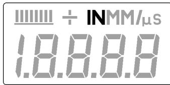
When the **IN** symbol is on, the **MMX-6 DL** is displaying a thickness value in inches. The maximum thickness that can be displayed is 19.999 inches.
