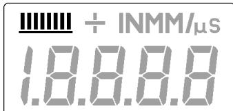
These eight vertical bars form the Stability Indicator. When the **MMX-6 DL** is idle, only the left-most bar and the underline will be on. While the gauge is taking a measurement, six or seven of the bars should be on. If fewer than five bars are on, the **MMX-6 DL** is having difficulty achieving a stable measurement, and the thickness value displayed will most likely be erroneous.
