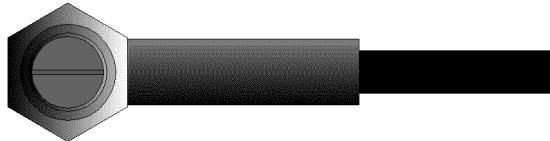
This is a bottom view of a typical transducer. The two semicircles of the wearface are visible, as is the barrier separating them. One of the semicircles is responsible for conducting ultrasonic sound into the material being measured, and the other semicircle is responsible for conducting the echoed sound back into the transducer. When the transducer is placed against the material being measured, it is the area directly beneath the center of the wearface that is being measured.
