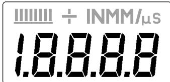
The numeric portion of the display consists of 4 complete digits preceded by a leading "1", and is used to display numeric values, as well as occasional simple words, to indicate the status of various settings. When the **MMX-6 DL** is displaying thickness measurements, the display will hold the last value measured, until a new measurement is made. Additionally, when the battery voltage is low, the entire display will begin to flash. When this occurs, the batteries should be replaced.
