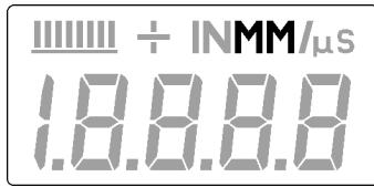
When the **MM** symbol is on, the **MMX-6 DL** is displaying a thickness value in millimeters. If the displayed thickness exceeds 199.99 millimeters, the decimal point will shift automatically to the right, allowing values up to 1999.9 millimeters to be displayed.
