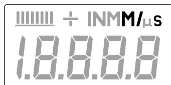
When the **IN** symbol is on, in conjunction with the **ms** symbol, the **MMX-6 DL** is displaying a sound-velocity value in **inches-per-microsecond**.
