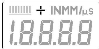
When the + symbol is on and blinking, this indicates that the **MMX-6 DL** is currently operating in **echo-echo ( Thru-paint/coating ) mode**.
