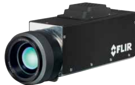
The FLIR G300a optical gas camera contains a cooled Indium Antimonide (InSb) detector that produces thermal images of 320 x 240 pixels.
