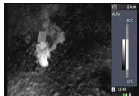
The FLIR G300a optical gas camera contains a cooled Indium Antimonide (InSb) detector that produces thermal images of 320 x 240 pixels.
